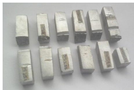
Figure 4.0: Impact Test Specimens After Fracture, (Materials Lab. FUTO, Owerri).
