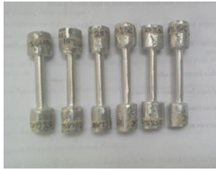
Figure 5.0: Tensile Test Specimens Before Fracture, (Materials Lab. ESUT, Enugu).
