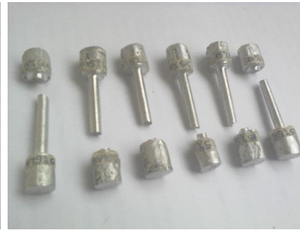
Figure 6.0: Tensile Test Specimens After Fracture, (Materials Lab. ESUT, Enugu).
