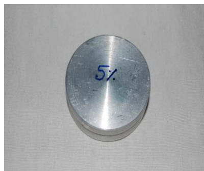
Figure 2.0: Hardness Test Sample Before Indentation, \phi 40mm, 15mm Thick Gauge, (Material Lab, FUTO, Owerri).
