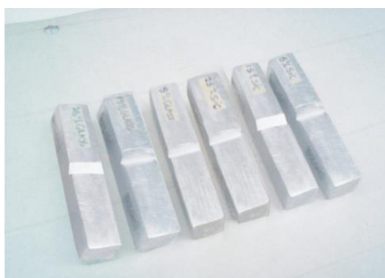
Figure 3.0: Impact Test Specimens Before Fracture (Materials Lab. FUTO, Owerri).
